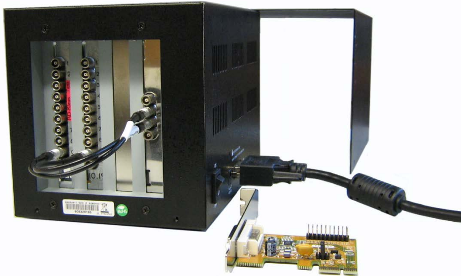
Figure 2.4: Two TDC8HP boards with clock card in a PCI2PCIe crate. A PCIe adapter card is shown on the lower right side.
